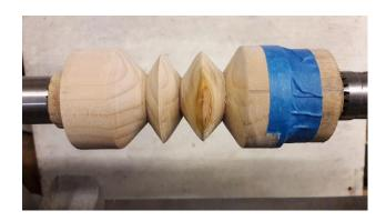
If the tenon on the tail piece is a bit loose it can be held in position with a piece of masking tape after lining up both pieces.
